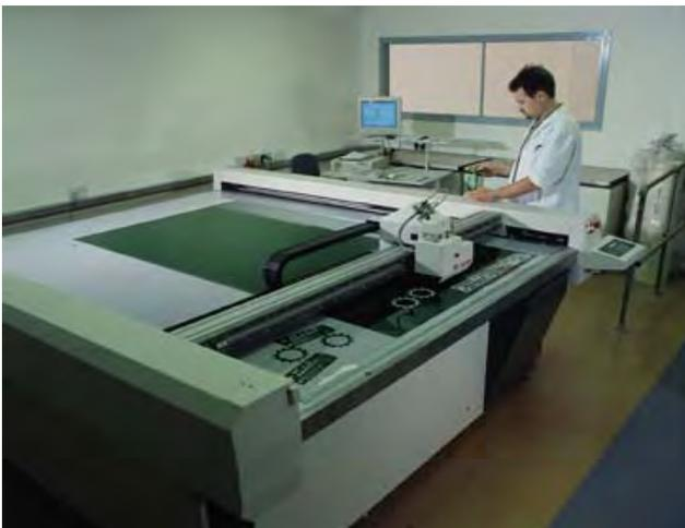
Parts are precision cut by our zero width X-Y CNC. Full CAD/CAM ability means we have no tooling charges (we can work directly from drawings or electronic files) and the delivery lead time is very short. EMI-ito15 can also be supplied in sheets or rolls, maximum standard web width = 760mm.
